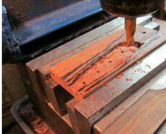
Use an air die grinder and a square-end burr to fine tune the recess. Try to fit the tang - locate any problem areas and then remove the wood at that spot. Make absolutely sure that once the tang fits into the recess that a pin can still pass through the tang & the corresponding hole. It doesn't, the problem is usually at the throat area. Align with pins and scribe that area - you will typically see what needs to go away.
