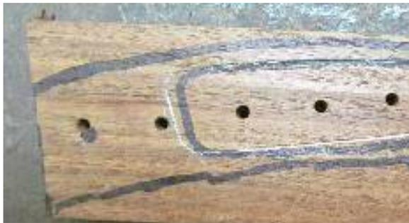
Use temporary pins to locate the tang correctly with the pins inserted through the tang and into the scale. Typically the pins will extend 1/2..3/4". Use a drill-press vise to clamp the pins and lock the complex together. Use a carbide scribe and trace the outline of the tang onto the scale. Repeat with a sharp pencil.
