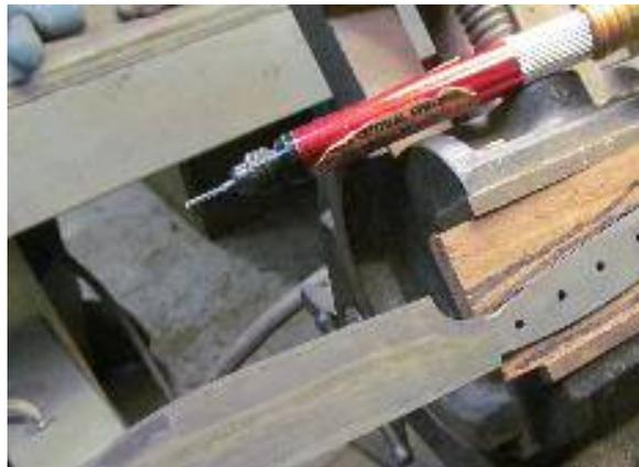
At this point, the tang will be recessed into the scale and half of the width of the spine is within the scale. If there is a dorsal-ventral taper, there will be air at the ventral aspect of the recess. That is what epoxy is for.
