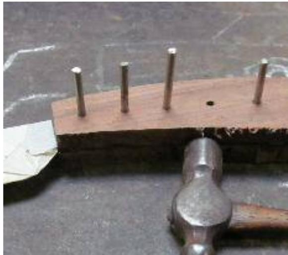
Butter the pins with epoxy and shove some epoxy into the holes on the other side of the handle. Go to the machinist vise and place the pins against the front jaw after positioning a backing board against the rear jaw. Use the vise to drive the pins - go slow and careful - do not bend the pins. You can drive all pins at once or each pin individually.
