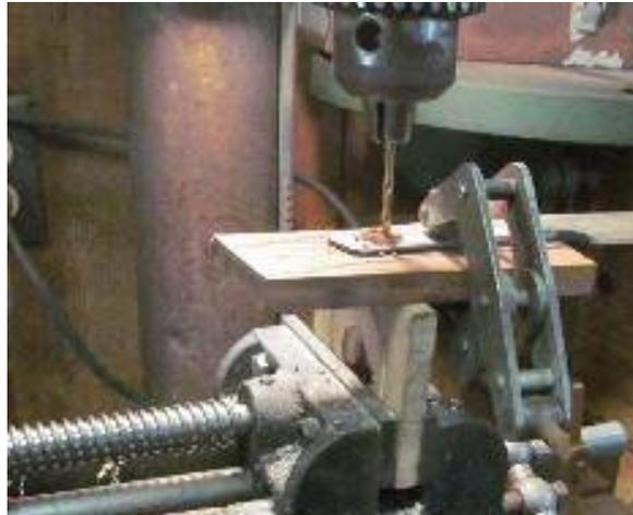
If the tang is short, lay out auxiliary holes from the tang to the pommel surface and drill the holes. A divider set can be used to transfer inter-pin distances.
