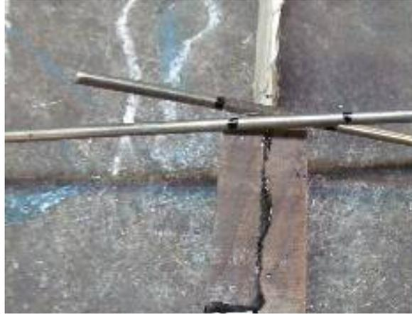
Shear the pins using a modified fence tool. Both ends are now distorted by the shear. Go to the grinder and grind a taper on one end of all pins.
